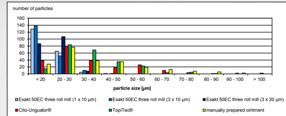
Fig. 2: Wool wax ointment with 10% salicylic acid; the particle size distribution of 200 particles in each sample was determined microscopically
