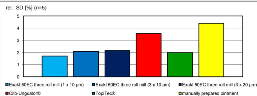
Fig. 1: Results of the homogeneity test with a formulation of 10% methylene blue in macrogol ointment
