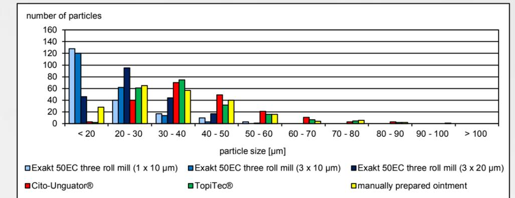
Fig. 5: Results of the stability test of wool wax ointment with 10 % salicylic acid (21 °C and 47% R.H. over 5 weeks)
